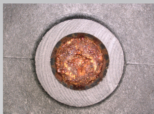
Figure 1: Corroded zinc-plated terminal connection at 20x magnification.
