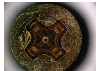
Figure 4: Brass terminal connection with dielectric grease at 50x magnification.
