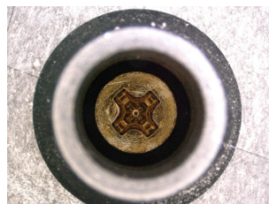
Figure 3: Brass terminal connection with dielectric grease at 20x magnification.
